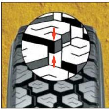
Minimum tread groove depths are specified for tire manufacturers under Federal Motor Vehicle Safety Standard 119, and for in-use applications by Federal Motor Carrier Safety Regulations, part 393.75. Under FMVSS 119, manufacturers must include tread depth indicators, commonly called "wear bars", in six locations evenly spaced around the circumference of a highway truck tire, so that they become visible when 2/32" of tread groove depth is remaining.
